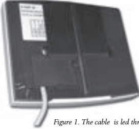
Figure 1. The cable is led through the outlet
